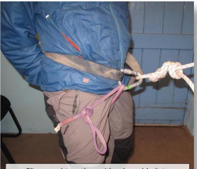
Sling used together with a broad belt to construct an improvised harness
